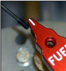
1. Determine (above) which side to insert the set screw that will key on the flat side of the selector valve.
