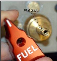
If your aircraft was designed to use the stock 'weather vane' lever with the tiny pointer pointing at the selected tank, then the set screw should go in the rear (wide side) of the lever.
