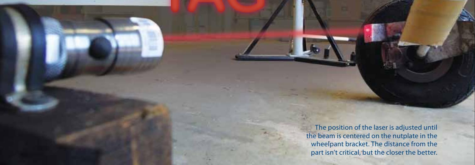
The position of the laser is adjusted until the beam is centered on the nutplate in the wheelpant bracket. The distance from the part isn't critical, but the closer the better.
