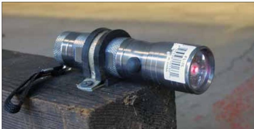
For security, the laser is mounted to a substantial wood block with a spare Adel clamp and a drywall screw.
