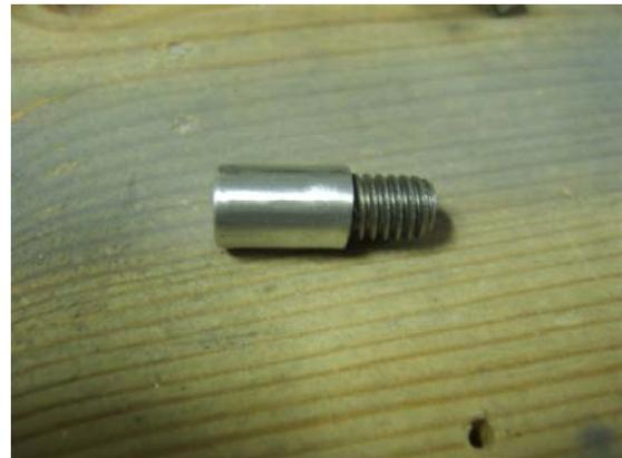
Drill #21 into roll pin holes in door handle gear. Tap for 10-32. Place gear onto handle assembly and align roll pin holes. Run tap into gear and handle assembly together. Insert 2 10/32 setscrews into gear until flush with the outside of the gear. The upper roll pin is replaced with this pair of setscrews and provides anti rotation protection. Also tighten two other setscrews for added security. When satisfied with fit, grind the tube of handle flush with gear top surface.
